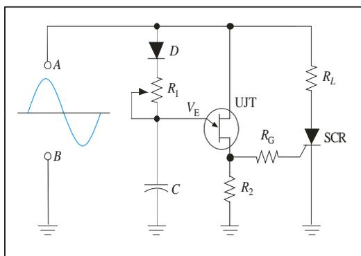
The UJT produces a fast, reliable current pulse to the SCR, so that it tends to fire in the same place every cycle.
