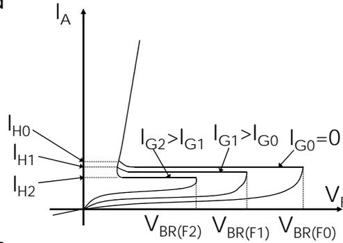
SCR characteristic curves for different  $I_G$  Values
