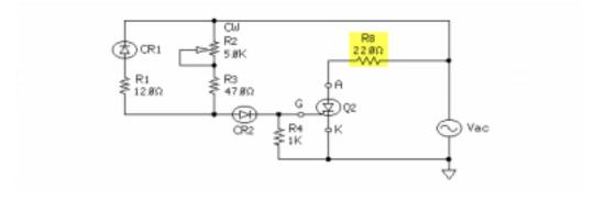
This circuit is a half-wave SCR phase control circuit. Power to the load (R8) can be controlled during the positive half of the input cycle.
