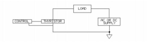
A **thyristor** is a semiconductor device. Electronically controlled switches use thyristors in industrial, military, aerospace, commercial, and consumer applications.
