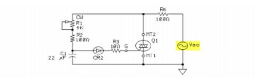
This is a half-wave triac circuit. The triac can be turned on only when Vac is positive.
