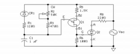
In this circuit, a UJT phase control is used with a half-wave rectifier.
