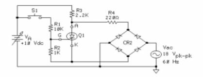
In this circuit, the SCR is a switch in series with load resistor R4. When S1 is closed,  $V_A$  supplies the gate trigger voltage and turns on the SCR. The SCR then acts like a closed switch, and a full-wave rectified waveform appears across R4.
