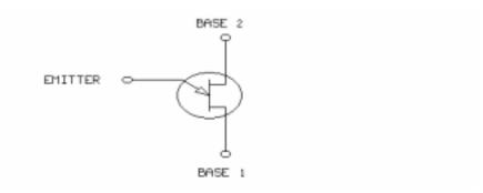
This is the symbol for a **unijunction transistor (UJT)**. The UJT has 1 PN junction and 3 terminals. In this unit, you will use the UJT to control the conduction angle of an SCR.
