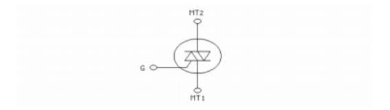
A triac is a 3-terminal **bidirectional** thyristor. A thyristor is any solid state switch. The triac is a thyristor that, unlike the SCR, is capable of conducting in either direction between its main terminals.
