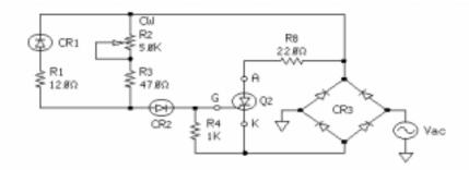
In this circuit, power to the load (R8) can be controlled on both halves of the input cycle. Therefore, the maximum power to the load is twice that of the half-wave circuit.
