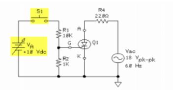
In this circuit, the SCR is a half-wave rectifier that is controlled by S1 and the dc supply  $(V_A)$ . The SCR turns off every negative half-cycle because the SCR becomes reverse biased.
