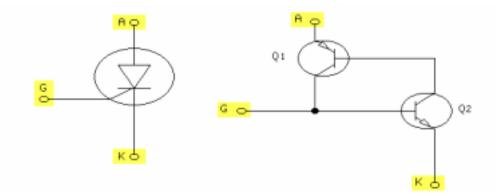
Internally, the SCR is similar to 2 cross-connected transistors. Above is the SCR symbol and its equivalent transistor circuit.
