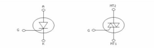
Similar to the SCR, a triac requires a minimum MT2 current to remain in conduction. This minimum current is the holding current.
