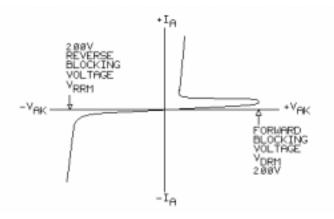
Shown are the voltage/current characteristics of an SCR with no gate current applied and with a forward and **reverse blocking voltage** rating of 200V.
